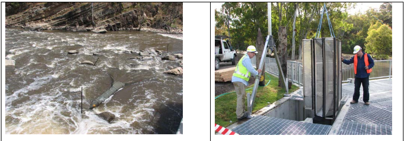
Figure 2: Equipment used to sample fish. Double winged fyke net (left); and purpose built trap (right)
